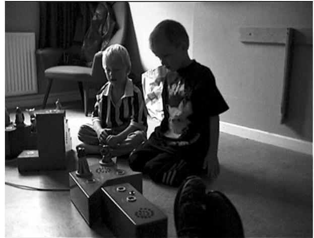
The physical set-up of the AudioTheatre consists of a “stage” with twelve contacts, and a number of painted backdrops. The “actors” are paper dolls cut in foam, placed on a plastic plugs with a small switch. Both paper dolls and backdrops have ID tags that can be read by the computer. The stage box contains a loudspeaker.
